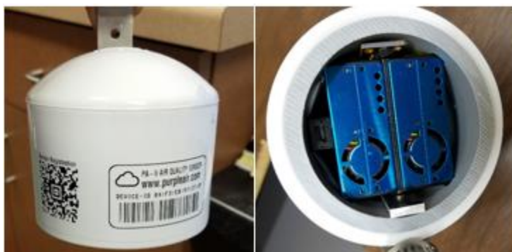
Figure 1: Individual purple air sensor unit containing two independent “Dual Laser” measurement sensors
