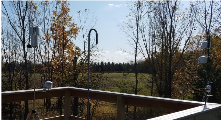
Figure 2: PurpleAir sensor collocated with T640 FEM at Appleton.
