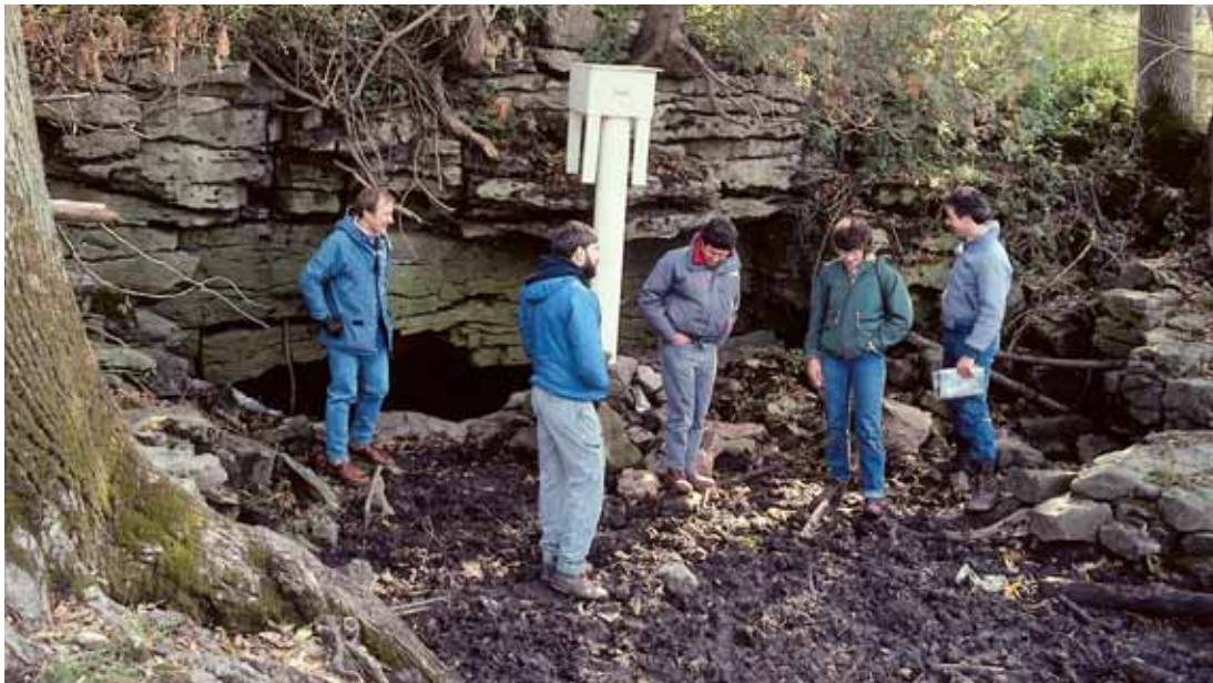
Groundwater research verified how quickly nearby contaminants washed pollution through a sinkhole into groundwater and seeped out to a discharge area. Pollution spreads wide, deep and quickly where the rock is fractured near the surface.
