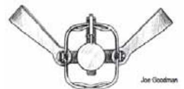
Live-restraining double longspring double-jaw foot-hold trap.
