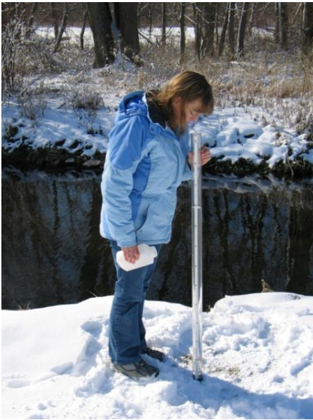
Figure 1: Transparency tube shaded by observer.
