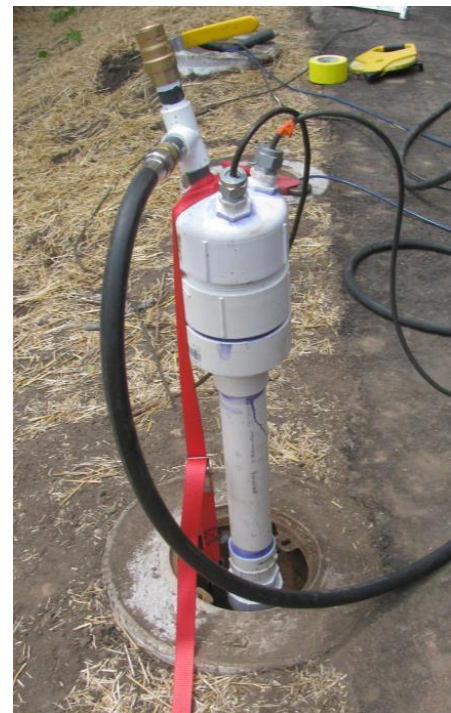
Pumping test at one of Madison's municipal wells, part of a WGRMP-funded study to enhance understanding of fractures and virus transport.
