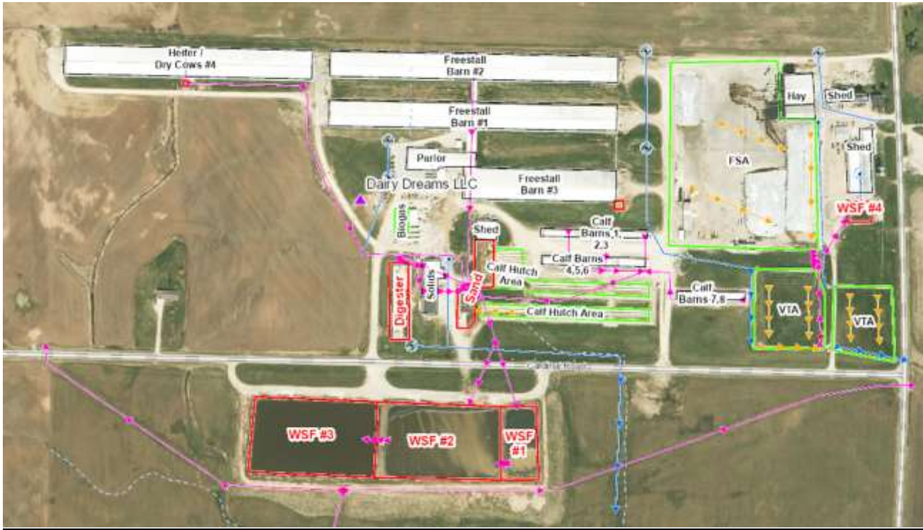
Aerial Map 1. The aerial map above illustrates the production site at Dairy Dreams LLC. The production site includes multiple animal barns, a calf hutch area, an anaerobic digester with natural gas production, solid separation, four liquid waste storage areas, one solid manure storage area, three permanent manure transfer locations, one feed storage area, two vegetated treatment areas, and a stormwater conveyance system. Buried waste transfer lines are represented by the pink arrows. Surface flow paths are represented by the yellow arrows. The stormwater conveyance system is represented by the blue arrows.
