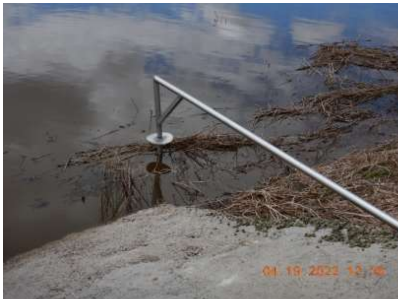
Photo 37. Permanent markers present within WSF 3. The MOL elevation is incorrect.
