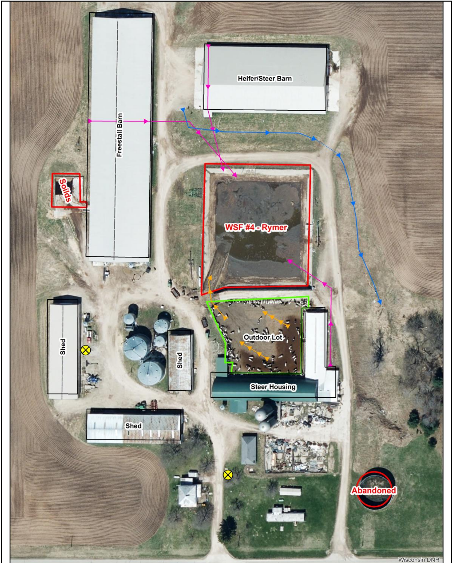
Site Overview Diagram (Rymer Farm: orange lines = potential runoff flow patterns, blue lines = stormwater flow, pink lines = waste transfer system, yellow circles indicate water supply well locations)
