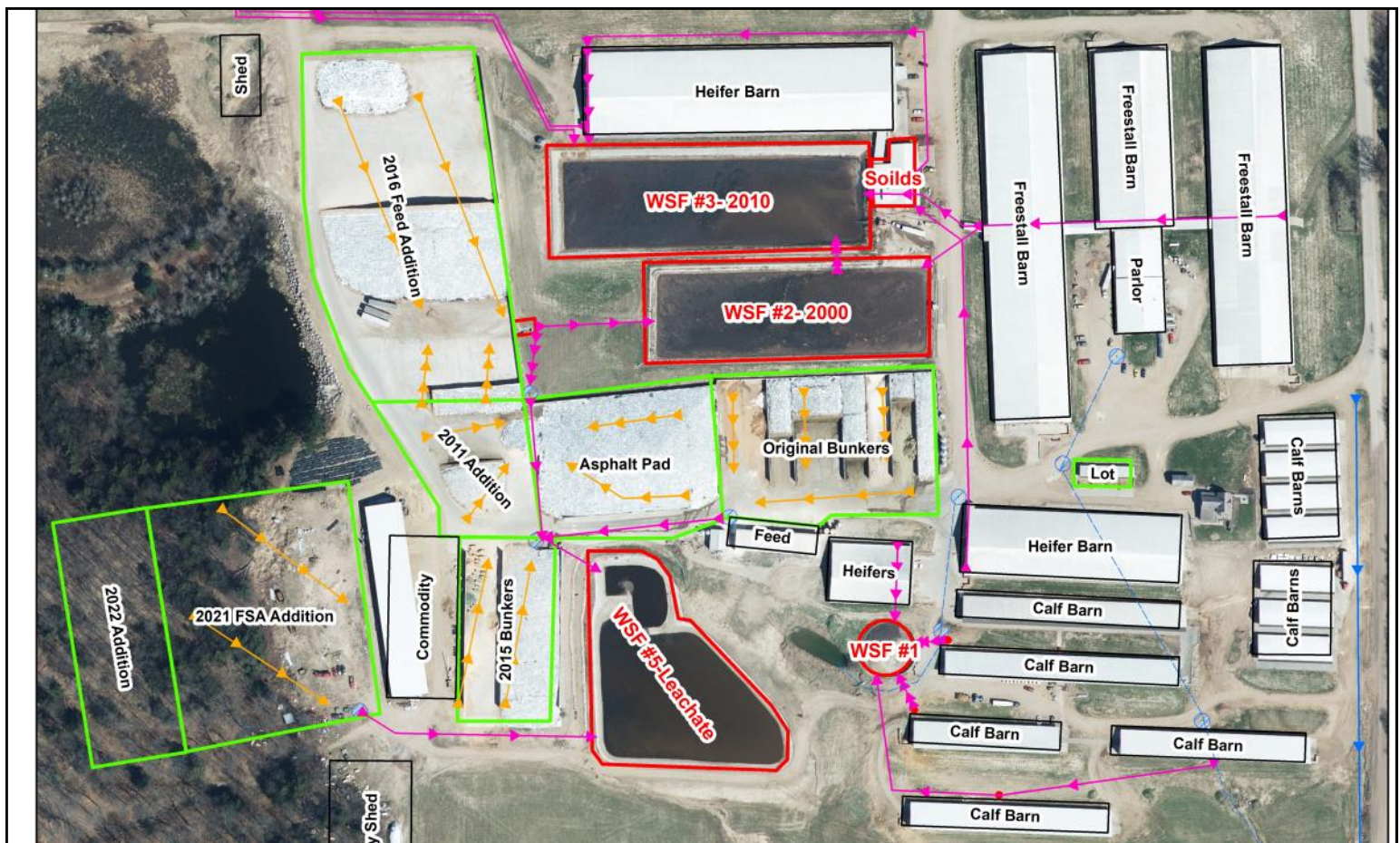
Site Overview Diagram (Main Farm South of County N: orange lines = potential contaminated runoff, blue lines = stormwater flow, pink lines = waste transfer system)
