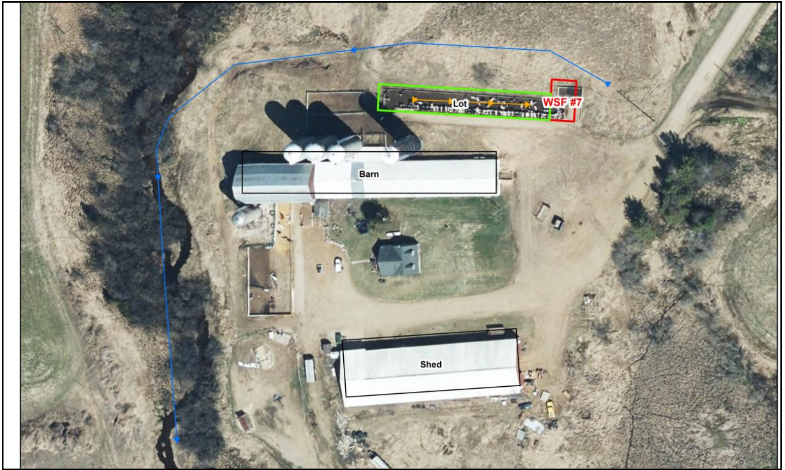
Site Overview Diagram (Pingel Farm: orange lines = potential contaminated runoff, blue lines= stormwater flow, pink lines= waste transfer system)
